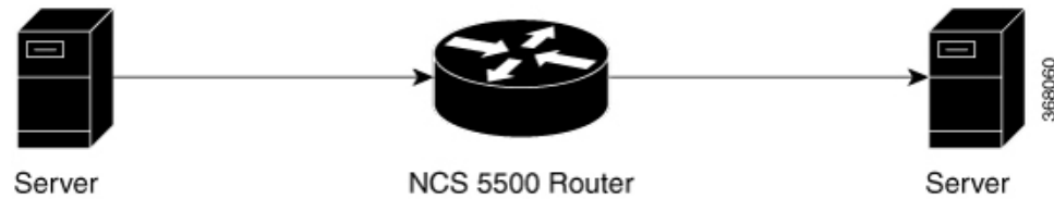
Figure 17: Topology for ERSPAN Egress Rate Limit
