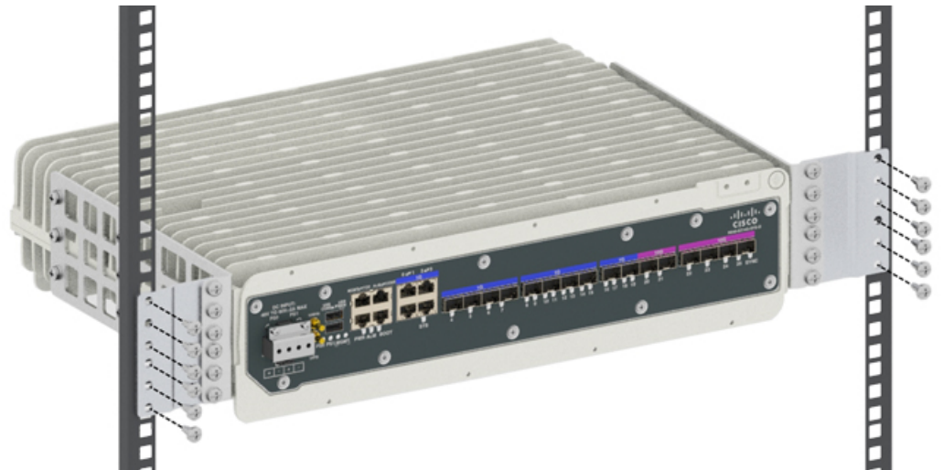
Figure 3: Install the Chassis in a 23-inch EIA Rack
