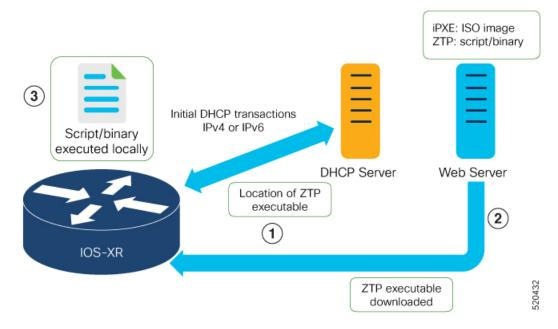
The ZTP process initiates when you boot the network-device with an IOS-XR image. The process starts only on the device that doesn't have a prior configuration.
