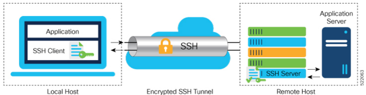
Figure 1: SSH Port Forwarding
