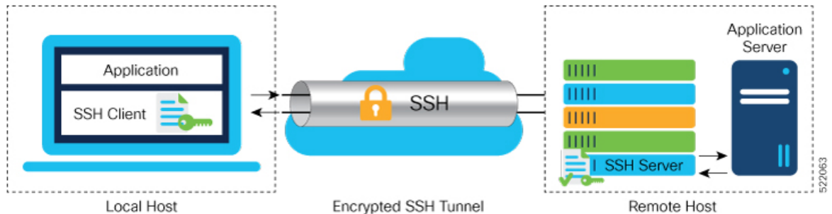
Figure 5: SSH Port Forwarding
