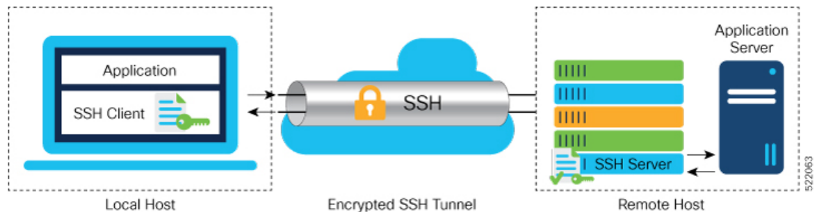
Figure 5: SSH Port Forwarding
