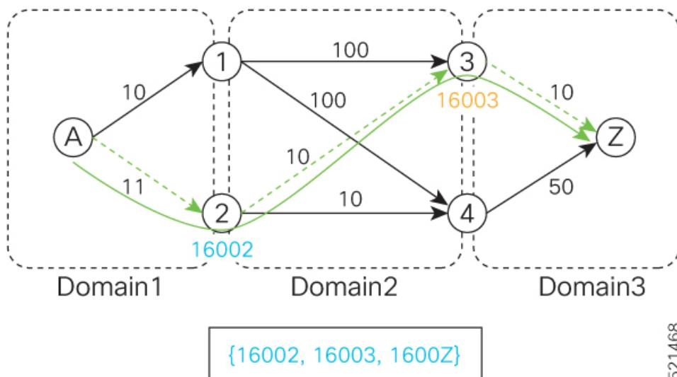
In this case, the optimized computed path from router A to router Z is 16002 > 16003 > 1600Z.
