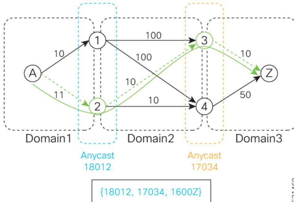
Using node SIDs, failures inside each domain (for example, links) benefit from fast TI-LFA convergence. However, failures of the ABR nodes would be dependent on SR-PCE reoptimization.
