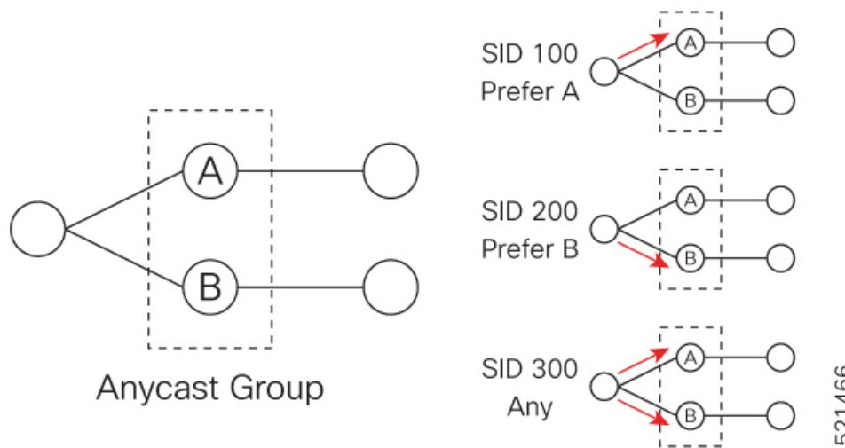
The Anycast replacement algorithm runs after an SR-TE path has been computed. It examines the prefix SIDs in the path and swaps them with Anycast SIDs that contain the same node. The new paths are checked against the original constraints and kept if suitable.
