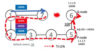
However, if nodes along the path do not converge at the same time, microloops can be introduced. For example, if Node2 converged before Node3, Node3 would send traffic back to Node2 as the shortest IGP path to Node6. The traffic between Node2 and Node3 creates a microloop.
