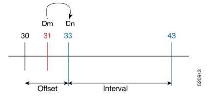
The link delay between 1-2 and 5-6 is normalized to 33.
