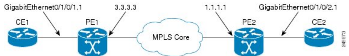
Figure 1: VPLS with BGP autodiscovery and BGP signaling
