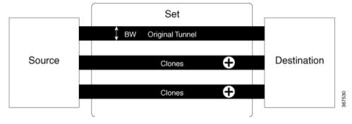
Merging is the process of removing a clone tunnel when the bandwidth demand decreases. If the bandwidth goes below the configured merge bandwidth in any one of the tunnels in the set, clone tunnels are removed.
