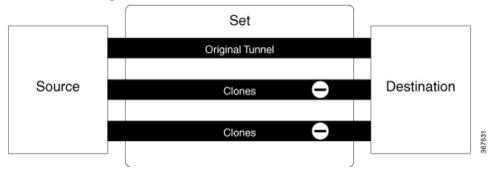
There are multiple ways to equally load-share the aggregate bandwidth demand among the tunnels in the set. This means that an algorithm is needed to choose the pair which satisfies the aggregate bandwidth requirements. You can configure a nominal bandwidth to guide the algorithm to determine the average bandwidths of the tunnels. If nominal bandwidth is not configured, TE uses the average of split and merge bandwidth as nominal bandwidth.
