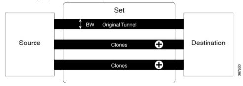
The following figure explains creating clone tunnels when the split bandwidth is exceeded.
