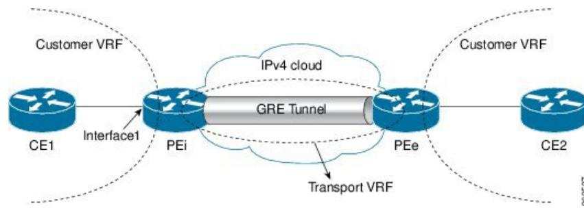
In the above topology, a GRE tunnel is configured in the core network, which is an IPv4 cloud. For packets entering through Interface1, the provider edge (PE) devices PEi and PEE are the tunnel head and tunnel exit respectively.
