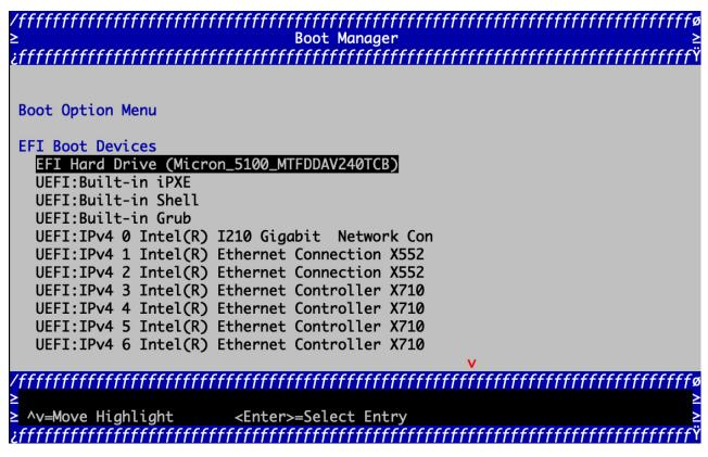
Step 5 If standby RP is present and it was stopped in step 2, boot the standby RP after the active RP starts to boot. From the boot options, select UEFI: Built-in iPXE and proceed with the boot-up procedure.
