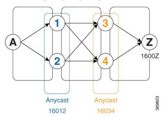
The Anycast SID aware path computation also provides resiliency. For example, if one of the ABRs (in this case, ABR 1) becomes unavailable or unreachable, the path from node A to node Z {16012,16034,1600Z} will still be valid and usable.
