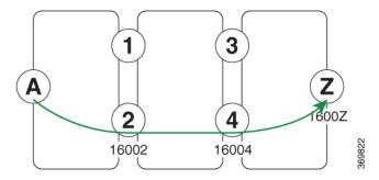
Assume that the computed path from node A to node Z traverses node 2 and node 4. This translates to SID list {16002, 16004, 1600Z} when node SIDs are leveraged to encode the path.
