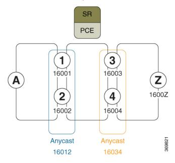
Consider the case where nodes A and Z are provider edge (PE) routers in the same VPN. Node A receives a VPN route with BGP next-hop to node Z. Node A resolves the SR path to node Z based on ODN behaviors with delegation of path computation to SR-PCE.
