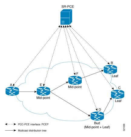
The tree computation algorithm on SR-PCE has been enhanced to detect a Bud node based on knowledge of the Leaf set, and to handle Leaf/Transit node transitions to Bud node. The role of the Bud node is also explicitly signaled in PCEP.
