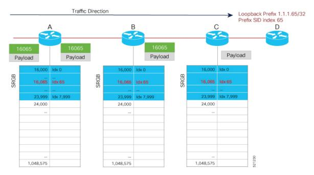
To keep the configuration simple and straightforward, we strongly recommended that you use a homogenous SRGB (meaning, the same SRGB range across all nodes). Using a heterogenous SRGB (meaning, a different SRGB range of the same size across nodes) is also supported but is not recommended.
