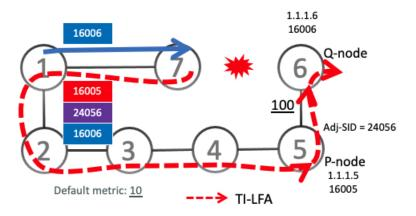
However, if nodes along the path do not converge at the same time, microloops can be introduced. For example, if Node2 converged before Node3, Node3 would send traffic back to Node2 as the shortest IGP path to Node6. The traffic between Node2 and Node3 creates a microloop.
