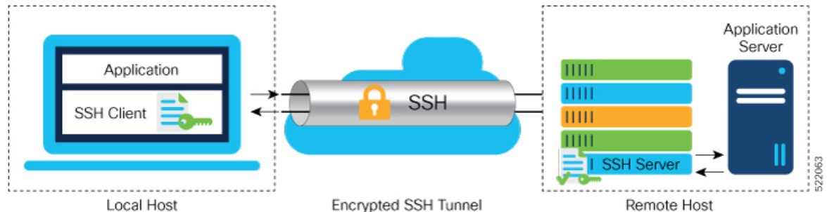
Figure 8: SSH Port Forwarding
