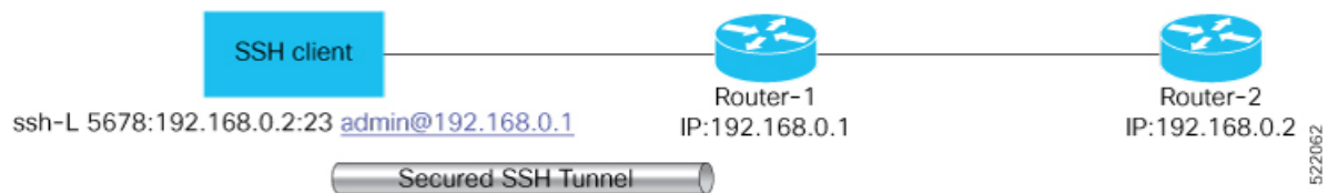
Figure 19: Sample Topology for SSH Port Forwarding
