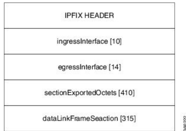
Figure 3: IPFIX 315 Export Packet Format
