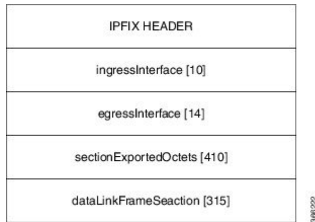
Figure 6: IPFIX 315 Export Packet Format
