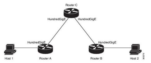
With a normal ping from Router A to Router B's HundredGigE interface, the source address of the ping packet would be the address of the outgoing interface; that is the address of the HundredGigE interface, (10.0.0.2). When Router B replies to the ping packet, it replies to the source address (that is, 10.0.0.2). This way, only the connectivity between the HundredGigE interface of Router A (10.0.0.2) and the 10gige interface of Router B (10.0.0.1) is tested.
