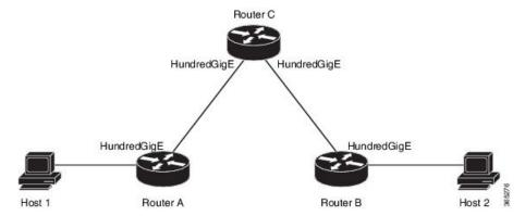
With a normal ping from Router A to Router B's HundredGigE interface, the source address of the ping packet would be the address of the outgoing interface; that is the address of the HundredGigE interface, (10.0.0.2). When Router B replies to the ping packet, it replies to the source address (that is, 10.0.0.2). This way, only the connectivity between the HundredGigE interface of Router A (10.0.0.2) and the 10gige interface of Router B (10.0.0.1) is tested.
