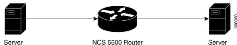
Figure 15: Topology for ERSPAN Egress Rate Limit
