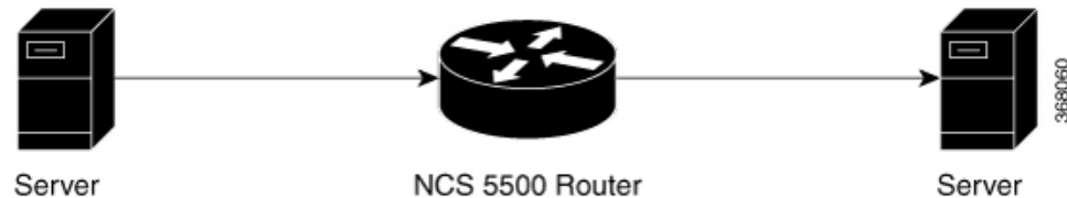
Figure 2: Topology for ERSPAN Egress Rate Limit
