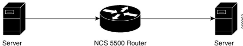
The encapsulated packet for ERSPAN is in ARPA/IP format with GRE encapsulation. The system sends the GRE tunneled packet to the destination box identified by an IP address. At the destination box, SPAN-ASIC decodes this packet and sends out the packets through a port. ERSPAN egress rate limit feature is applied on the router egress interface to rate limit the monitored traffic.
