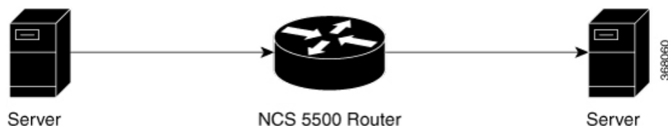
Figure 2: Topology for ERSPAN Egress Rate Limit
