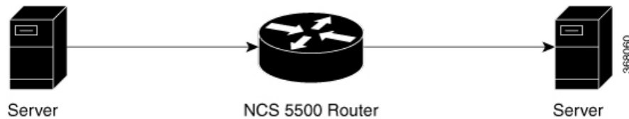
Figure 4: Topology for ERSPAN Egress Rate Limit
