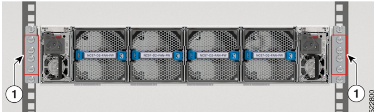
Figure 75: Remove Screws from the Slider Bracket - Port Side Exhaust Configuration
