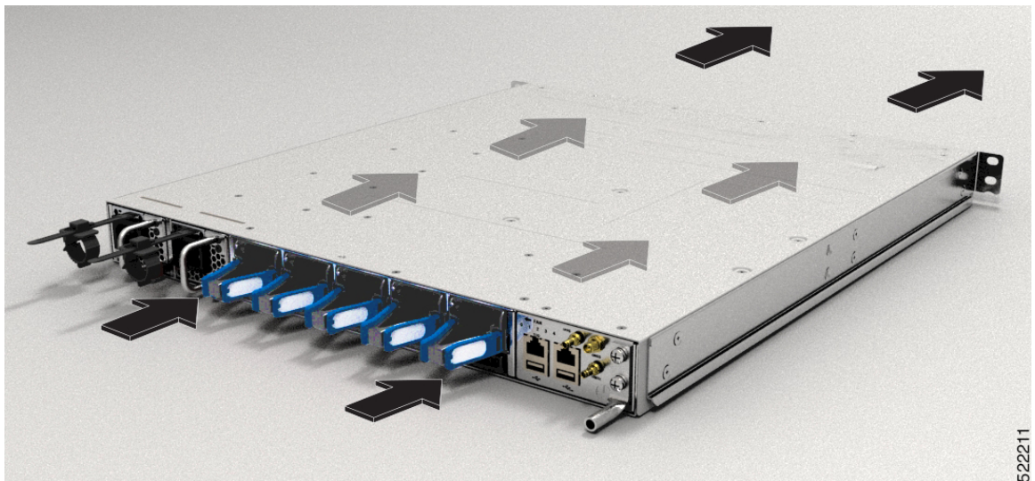
Figure 28: Port Side Exhaust Airflow Direction
