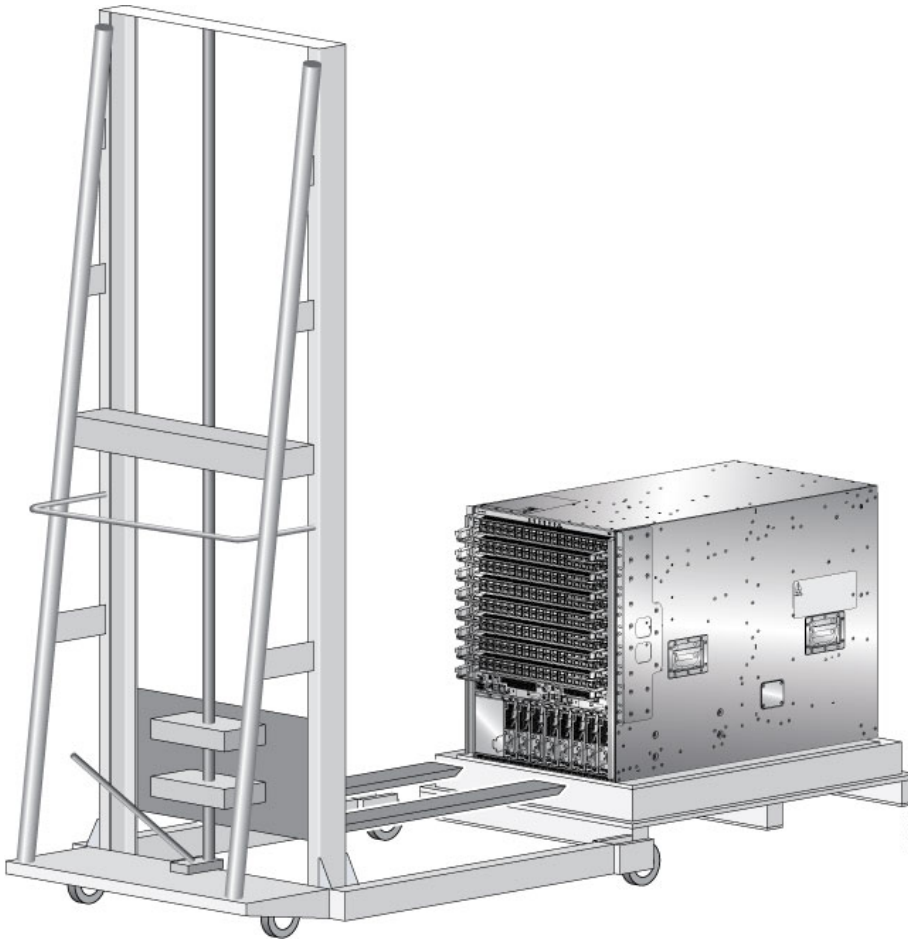
Figure 3: Align the Lifting Device In Front of the Chassis on the Pallet
