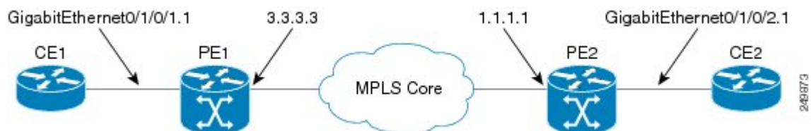
Figure 10: VPLS with BGP autodiscovery and BGP signaling
