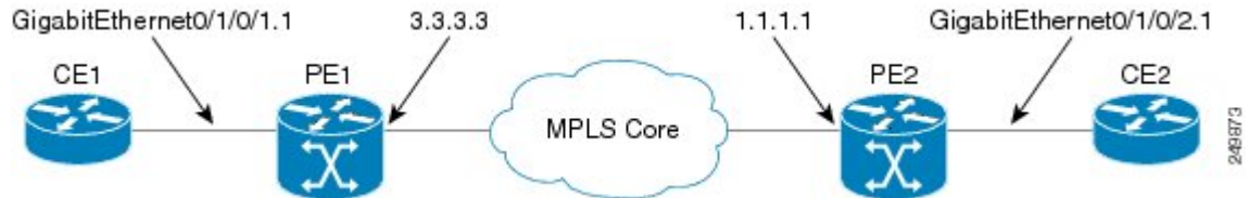
Figure 10: VPLS with BGP autodiscovery and BGP signaling
