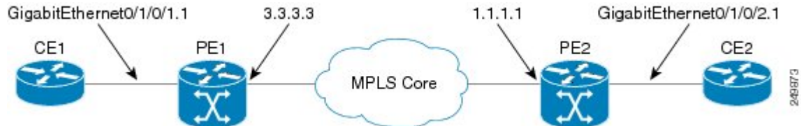
Figure 10: VPLS with BGP autodiscovery and BGP signaling
