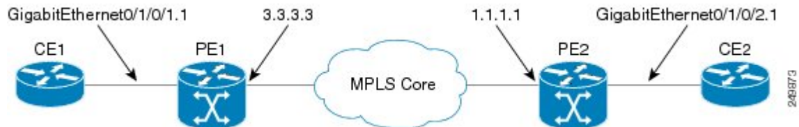
Figure 10: VPLS with BGP autodiscovery and BGP signaling
