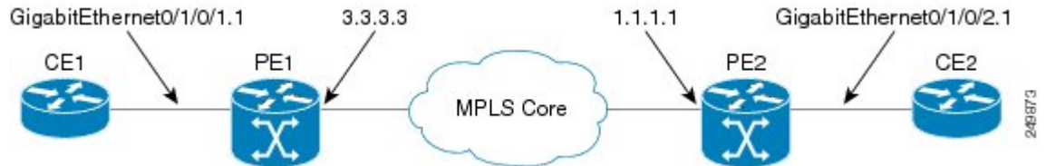
Figure 12: VPLS with BGP autodiscovery and BGP signaling
