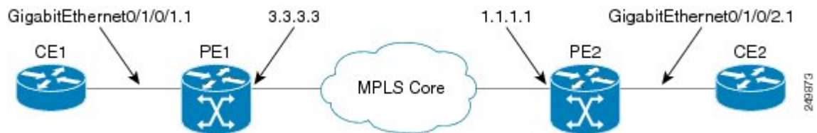
Figure 15: VPLS with BGP autodiscovery and BGP signaling
