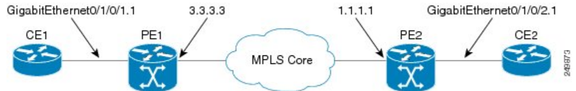
Figure 7: VPWS with BGP autodiscovery and LDP signaling
