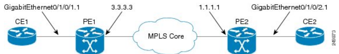
Figure 6: VPWS with BGP autodiscovery and BGP signaling
