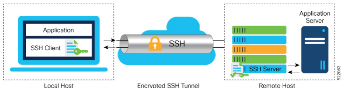
Figure 1: SSH Port Forwarding
