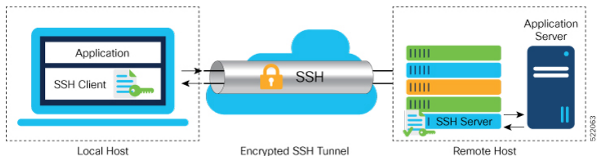
Figure 1: SSH Port Forwarding
