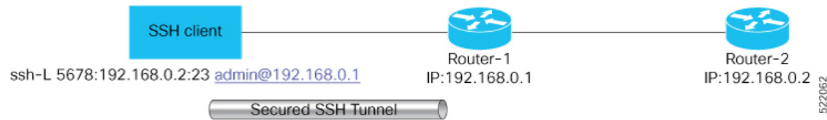
Figure 2: Sample Topology for SSH Port Forwarding
