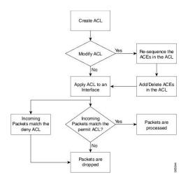
**Note** If there is no match to either permit or deny the packets, then the default action is to drop the packet.
