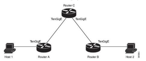
With a normal ping from Router A to Router B's TenGigE interface, the source address of the ping packet would be the address of the outgoing interface; that is the address of the TenGigE interface, (10.0.0.2). When Router B replies to the ping packet, it replies to the source address (that is, 10.0.0.2). This way, only the connectivity between the TenGigE interface of Router A (10.0.0.2) and the 10gige interface of Router B (10.0.0.1) is tested.
