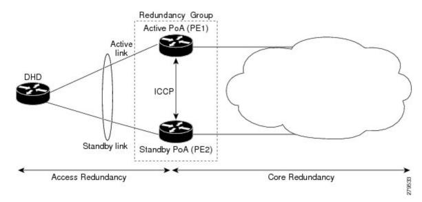
Figure 2: mLACP/ICCP Redundancy Model
