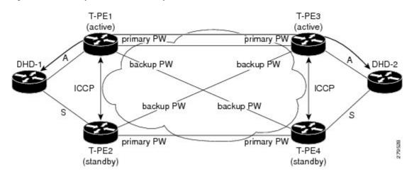
Figure 6: VPWS two-way Pseudowire Redundancy
