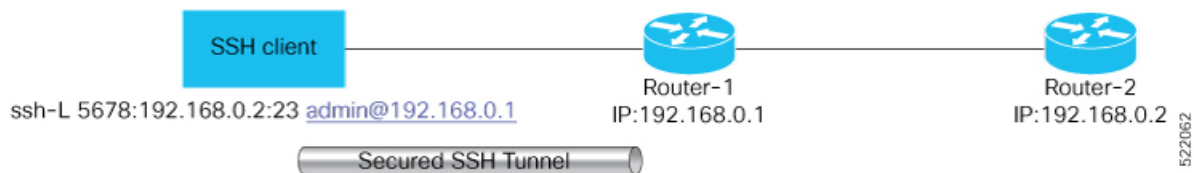
Figure 17: Sample topology for SSH port forwarding
