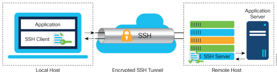
Figure 16: SSH port forwarding
