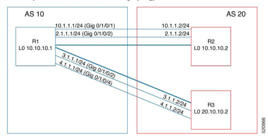
In this example, BGP-EPE peer SIDs are allocated from the default SRLB label range (15000 - 15999). The BGP-EPE peer SIDs are configured as follows:
