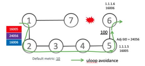
After the RIB update delay timer expires, the microloop-avoidant path is replaced with regular forwarding paths; traffic now natively follows the post-convergence path.
