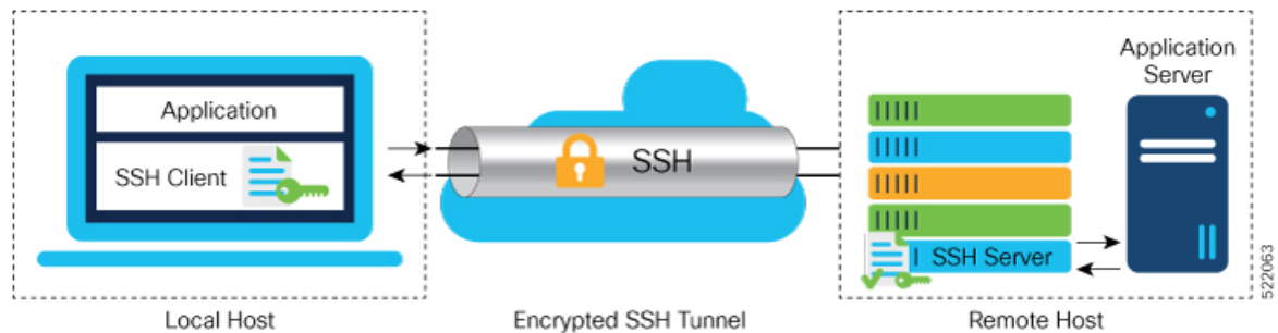
Figure 15: SSH Port Forwarding
