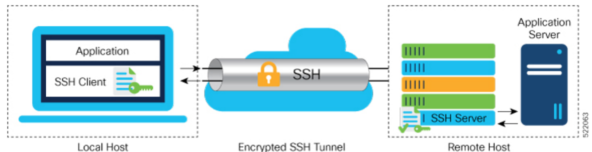
Figure 1: SSH Port Forwarding
