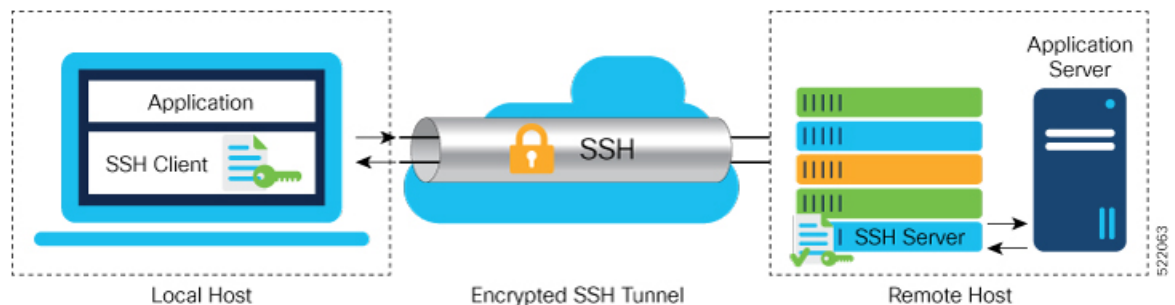
Figure 2: SSH Port Forwarding
