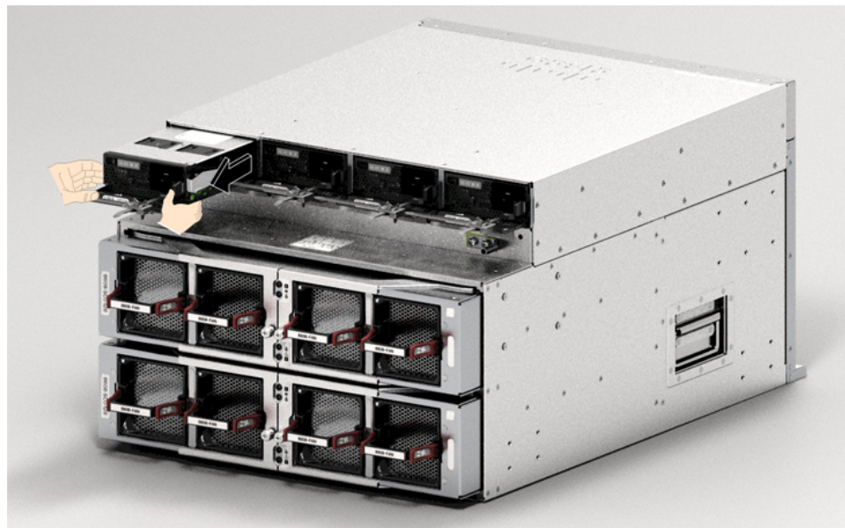
Figure 13: Slide the PSU Out
