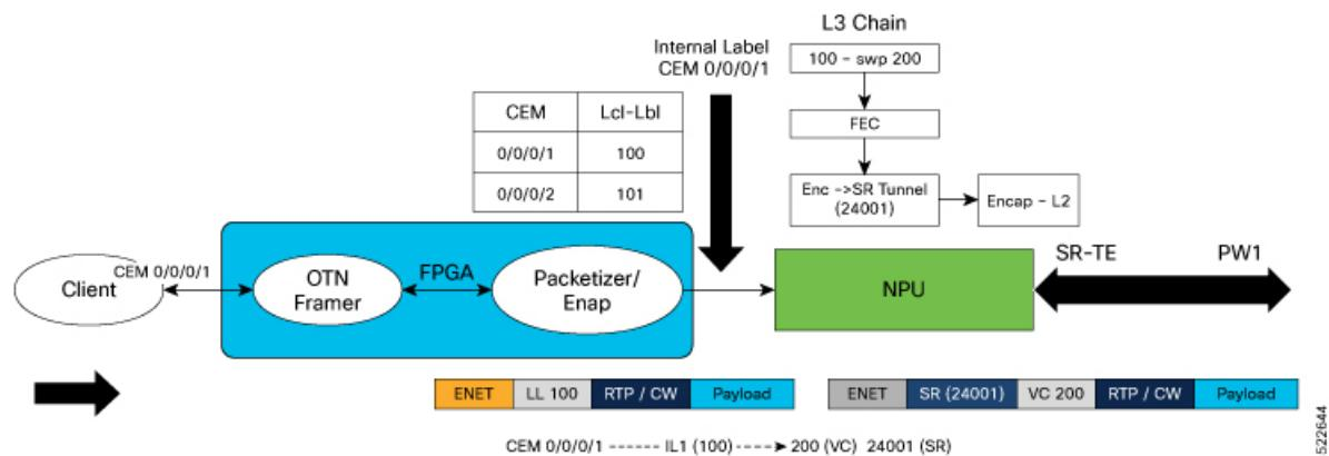
In the diagram, traffic from client may be of any port mode like FC, OTN, SDH, SONET, or Ethernet. Field Programmable Gate Array (FPGA) acts as a forwarding block. FPGA sends the traffic from the client towards NPU with an assigned internal local label.
