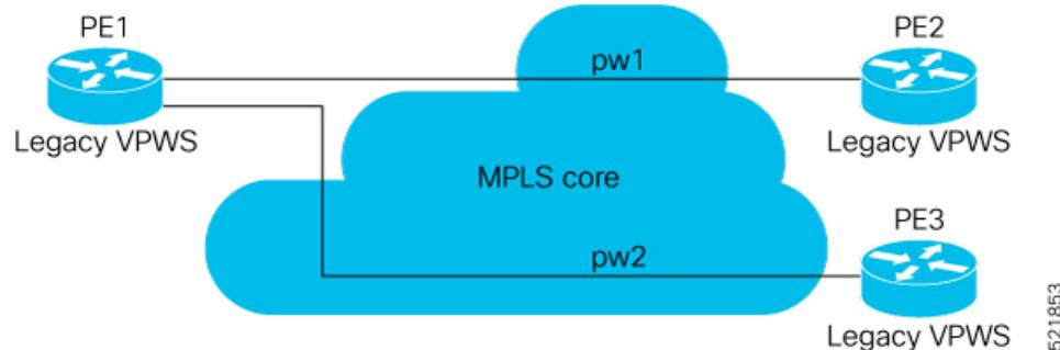
In this topology, PE1, PE2, PE3 are provider edge devices in the MPLS network and the legacy VPWS cross-connects are up and running between PE1, PE2, and PE3.
