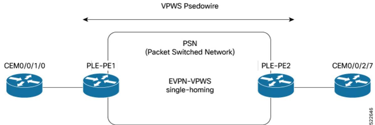
In this topology, CEM interfaces are connected to PLE interfaces. The PLE interfaces, PE1 and PE2, are connected through EVPN-VPWS single homing. The PLE interface can be: Ethernet, OTN, FC, or SONET/SDH.
