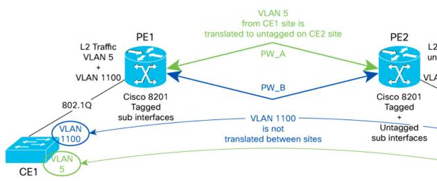
Let's understand the feature using this sample topology, in which the P2P L2VPN service is deployed between the two CE devices.
