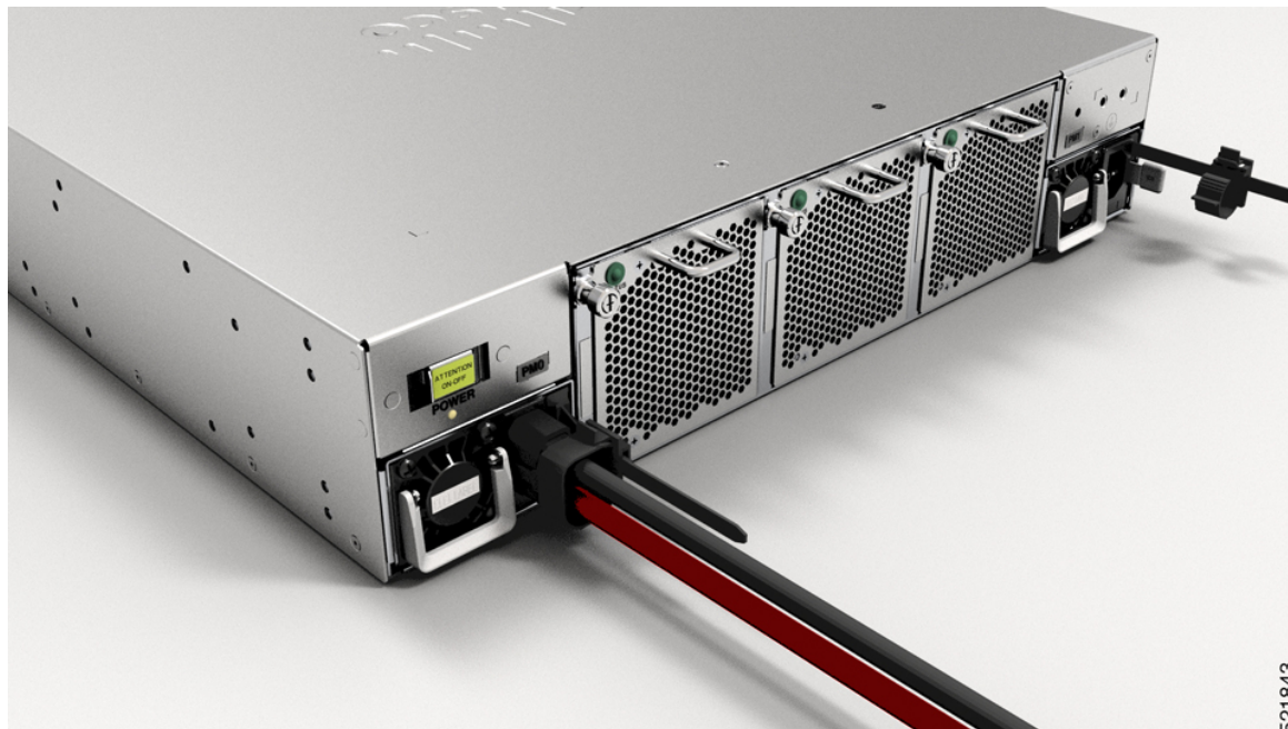
Figure 71: Cisco ASR 9903 DC Power Source Cabling Scheme for a Single DC Power Module
