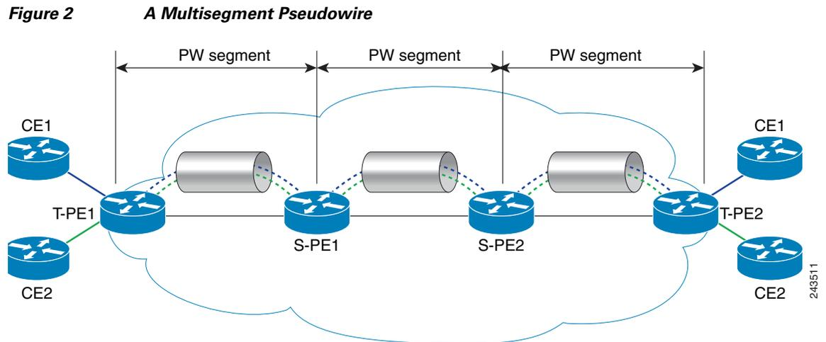
The end routers are called terminating PE routers (T-PEs), and the switching routers are called S-PE routers. The S-PE router terminates the tunnels of the preceding and succeeding PW segments in an MS-PW. The S-PE router can switch the control and data planes of the preceding and succeeding PW segments of the MS-PW. An MS-PW is declared to be up when all the single-segment PWs are up. For more information, see the [L2VPN Pseudowire Switching](#) document.
